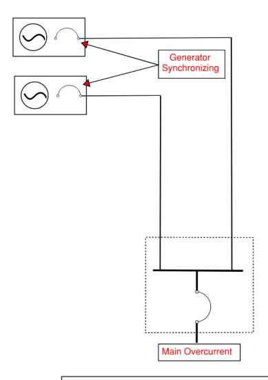
If the generator synchronizing is being done within the generators, both generators must terminate into a single overcurrent device. The single overcurrent device shall be sized for the combined sum of the generators.
